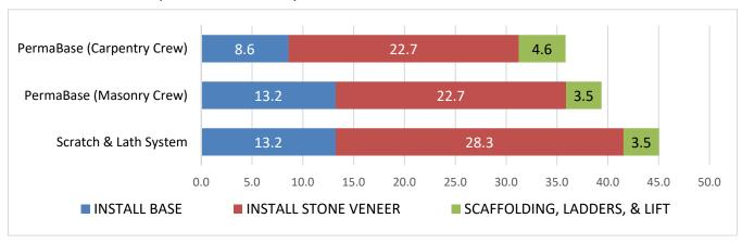
This study demonstrated that using PermaBase with LATICRETE® MVIS Veneer Mortar has the potential of saving 14% to 20% on the total installation time of homes.
